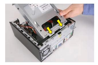
**9** Replace the two optical drive cage screws.
